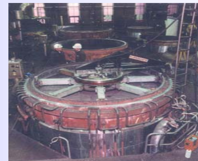
Ammonia Burner (head removed for refurbishment)
